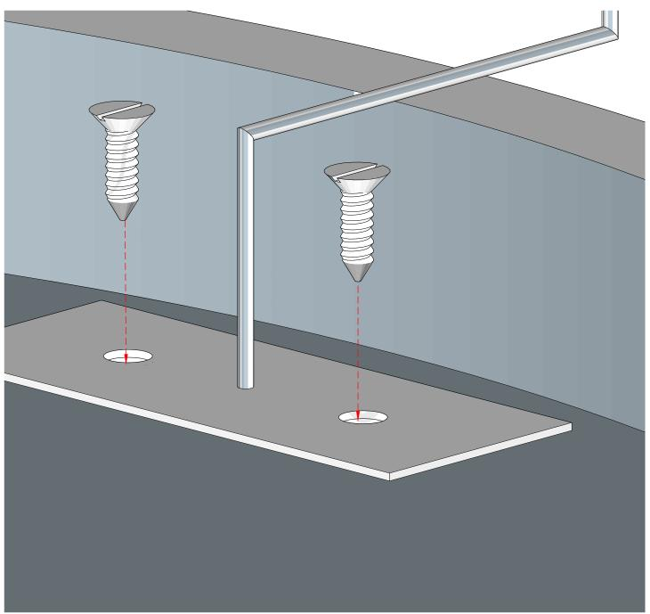
Step 1: Place Mounting Bracket near the edge of the pan. The hook should be centered above the pan.
