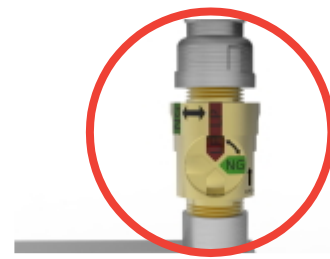
Figure 10.1 – Locating orifice for cleaning
